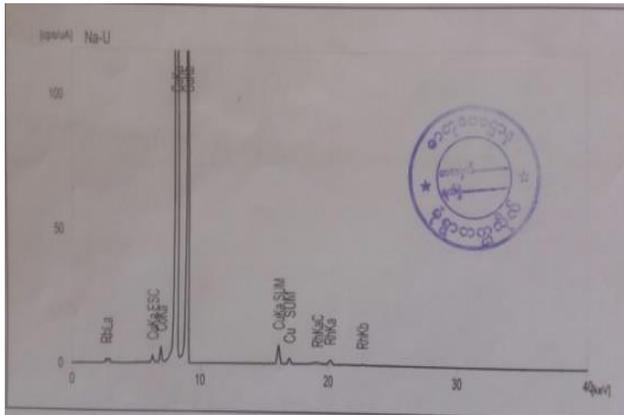
Fig .1 EDXRF spectrum of CuO nanoparticles
