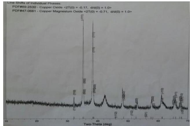
Fig .3 XRD spectrum of CuO nanoparticles
