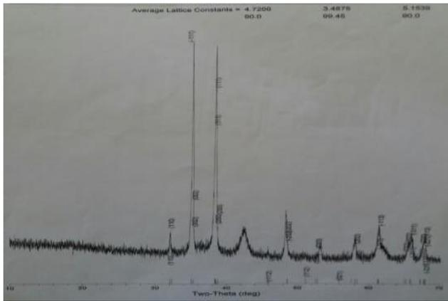
Fig. 4 XRD Spectrum of CuO nanoparticles
